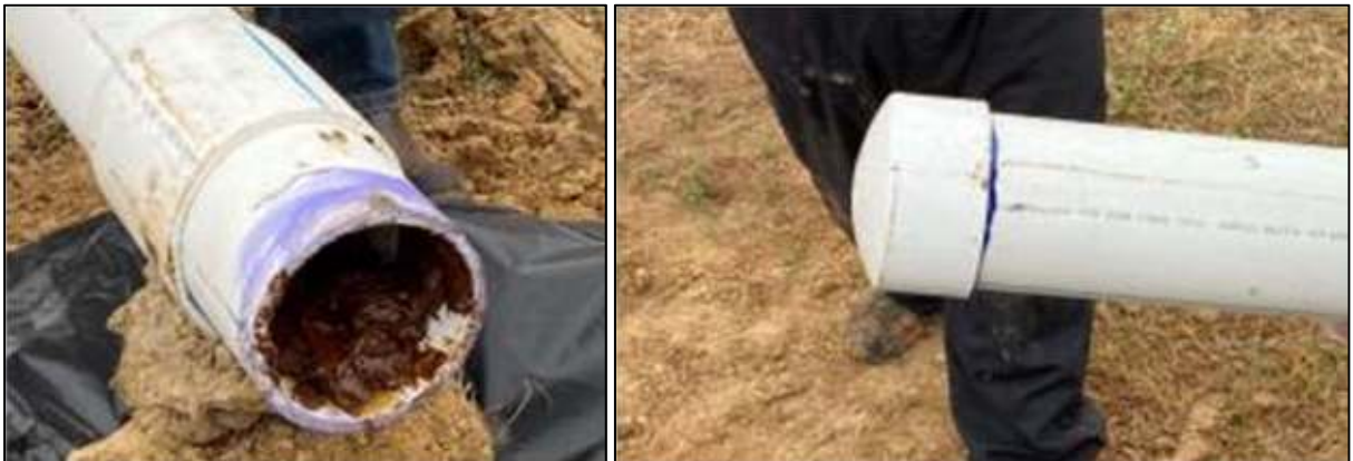
Figure 3.5 Weathered Macondo ("Juniper") oil placed and sealed at the bottom of a 15-foot (5-m) pipe
