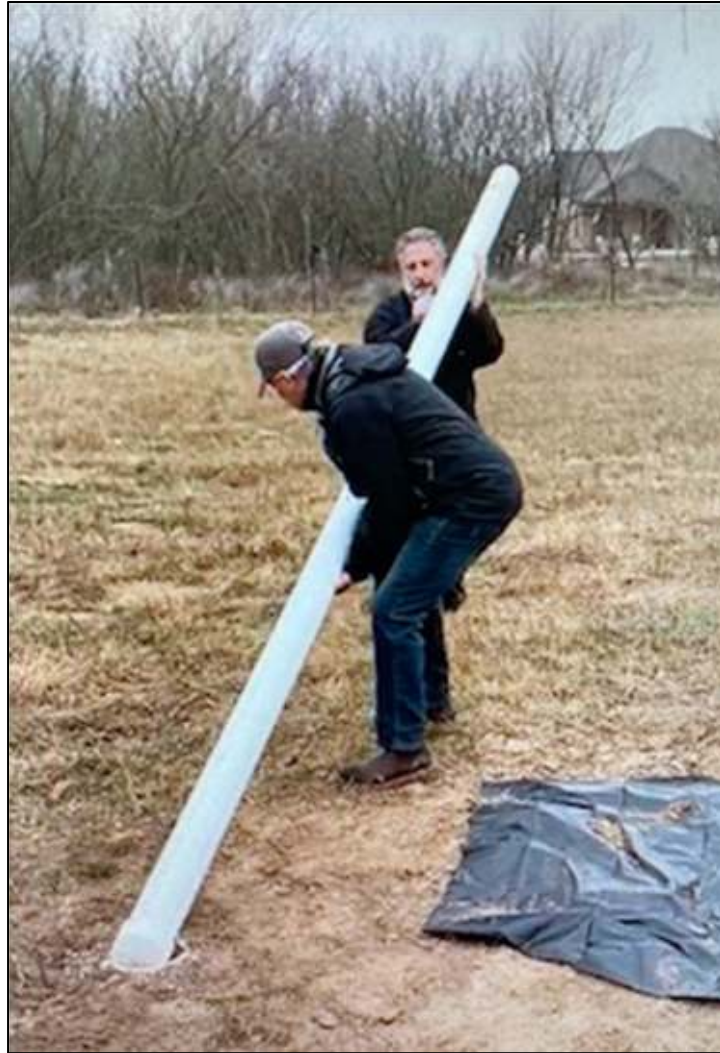
Figure 3.6 Insertion of the 15-foot (5-m) inner pipe with loaded target
